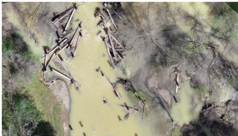
Aerial image of a Dry Creek Habitat Enhancement feature following a high-flow event.
